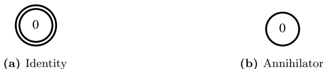
Figure 3.11: The identity and the annihilator for the concatenate operation. The language of the identity graph is the empty string \{\epsilon\} . The language of the annihilator graph is the empty set \{\} .
